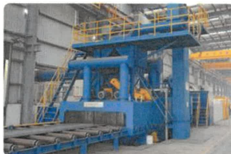
Shot Blasting Processing
