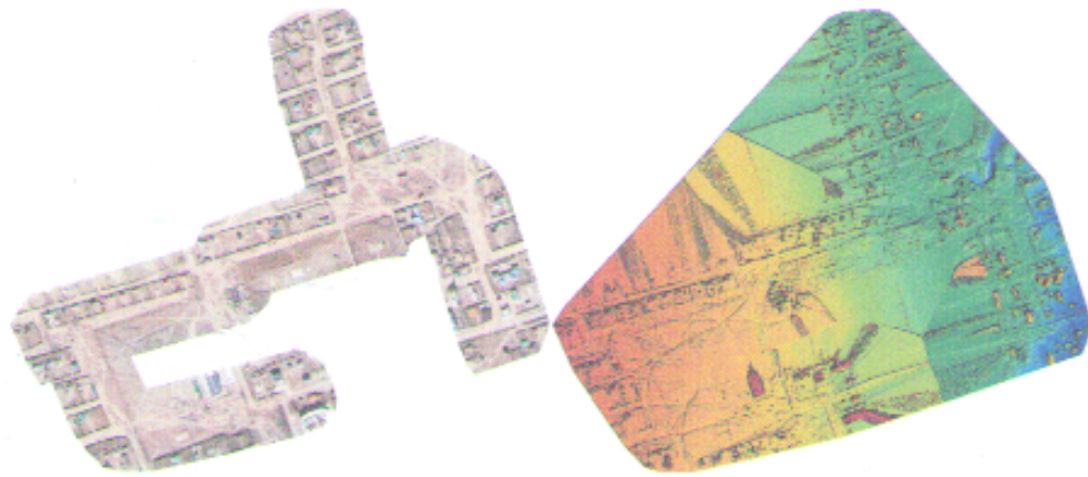
Figure 1: Orthomosaic and the corresponding sparse Digital Surface Model (DSM) before densification.
