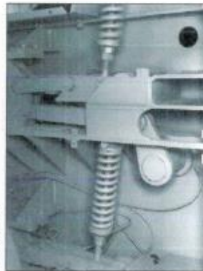
Tramp protection on upper & lower stages is provided by Automatic Toggle Mechanisms.
